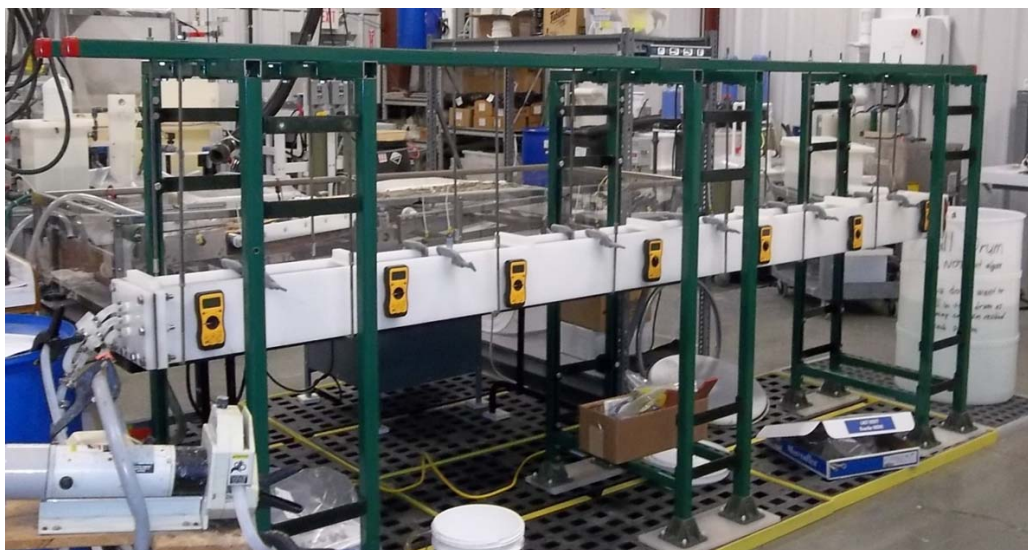
Figure 8: 12 ft x 5 in x 5 in flow channel constructed at Faraday for continuous processing of bioalgae pond solution.
