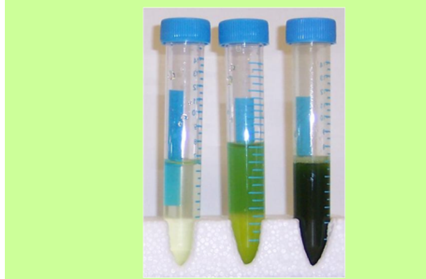
Figure 5. Demonstration of the ability to purify pond water (left), initial solution (middle) and concentrated algae (right) using the FARADAYIC SM ElectroConcentration Process.
